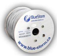
BlueStorm 23AWG Cat6A 500MHz UTP Solid Bare Copper Ethernet Cable is high-speed cabling specifically designed for use in 10GBase-T (10Gbps) indoor network environments. Constructed using 23AWG solid pure bare copper conductors with a PVC jacket and a cross separator, it exceeds TIA/EIA 568-C.2 standards and it is safe for use in the Riser spaces of commercial class buildings. This cable is RoHS compliant.
